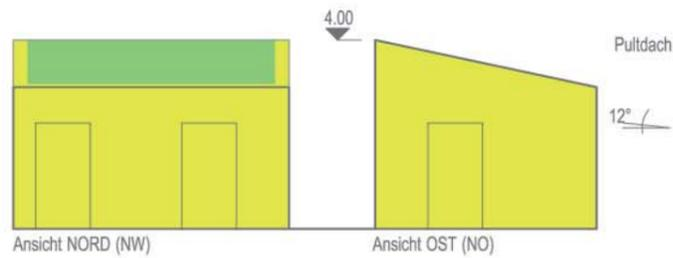
Green roof impossible due to the high roof angle
